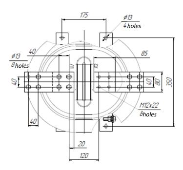
**Version F** – transformer with switching over on the primary winding.
